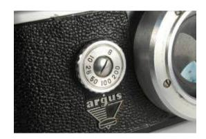
The M/F switch position for flash bulb synchronization was on top of the body to the right of the hot shoe for the majority of the production run. The switch was moved to the back of the camera on the right side of the viewfinder at about serial number 61000.
