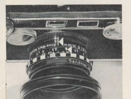
If the lens markings are not readily visible from the top of the camera—a convenience, not a necessity—the following adjustment may be made with a small jeweler's screwdriver. If you do not desire to make this adjustment, your local Dealer can do it for you.
